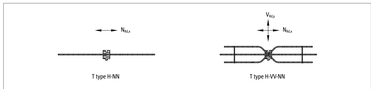
Fig. 219: Schöck Isokorb® T type H: Type selection
