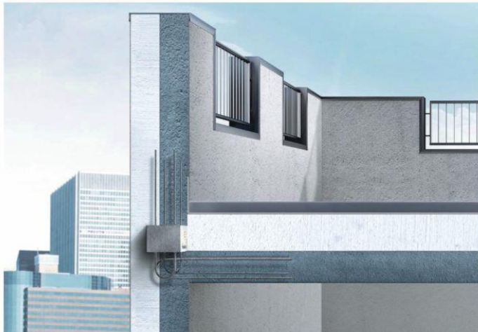
Schöck Isokorb type AXT shown in position. Image: Schöck Ltd.
