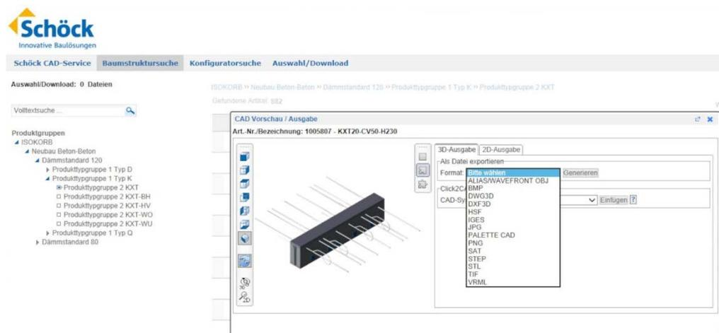
***The CAD service portal enables easy BIM-compliant Isokorb planning***
