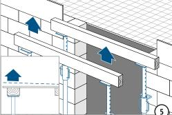
Step formwork in accordance with work plan.
