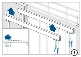
Step formwork in accordance with work plan.
