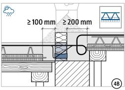
Be sure to fill the compression joint with in-situ concrete! Joint width ≥ 100 mm.
