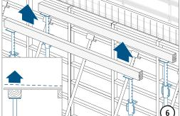
Step formwork in accordance with work plan.
