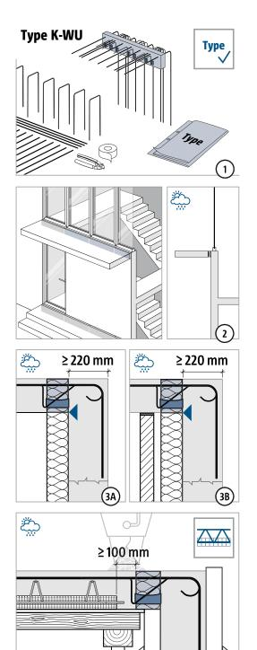
Be sure to fill the compression joint with in-situ concrete! Joint width ≥ 100 mm.
