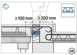
Be sure to fill the compression joint with in-situ concrete! Joint width ≥ 100 mm.
