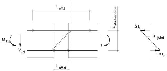
Fig. 52: Model for determining the bending deformation in the joint
