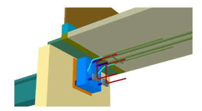
SOLIDO model of KS14 connection. The slab is omitted for clarity.
